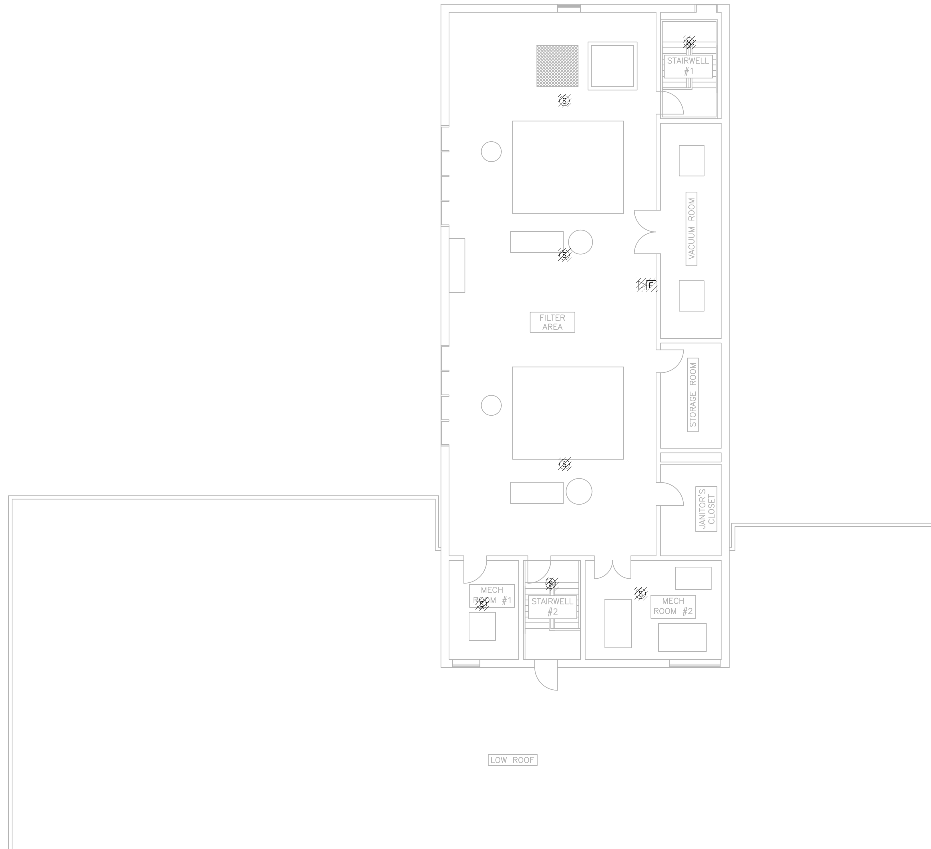
2ND FLOOR - DEMOLITION PLAN SCALE: 1/8" = 1'
