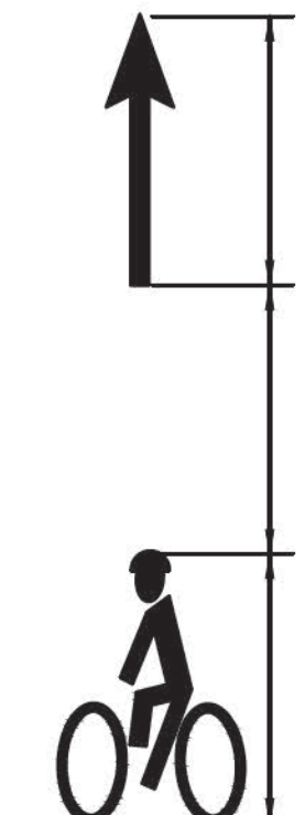
BICYCLE LANE MARKING DETAIL
