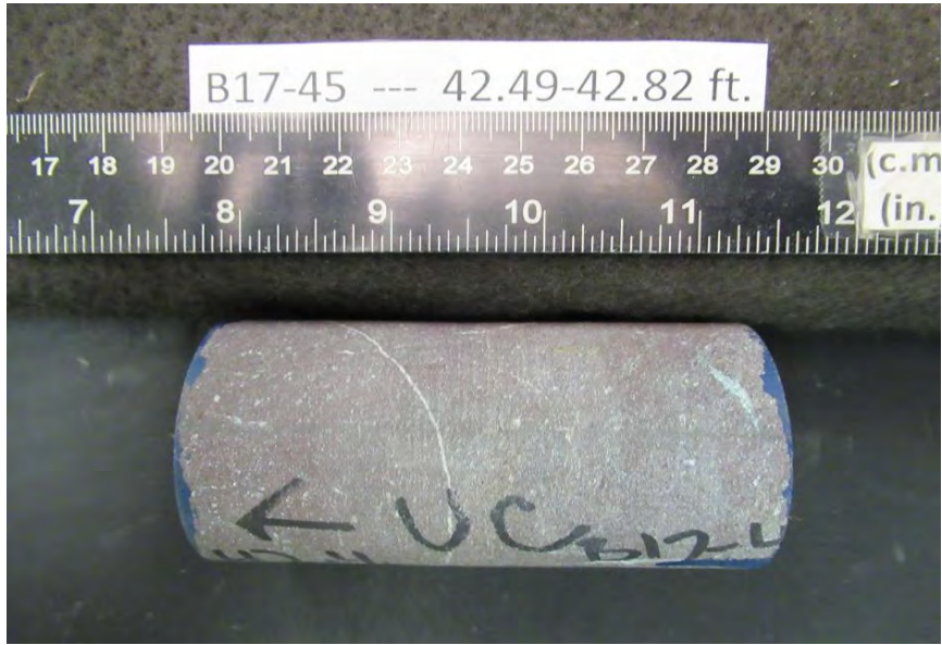
After cutting and grinding
