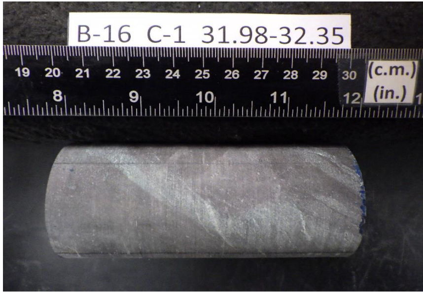
After cutting and grinding
