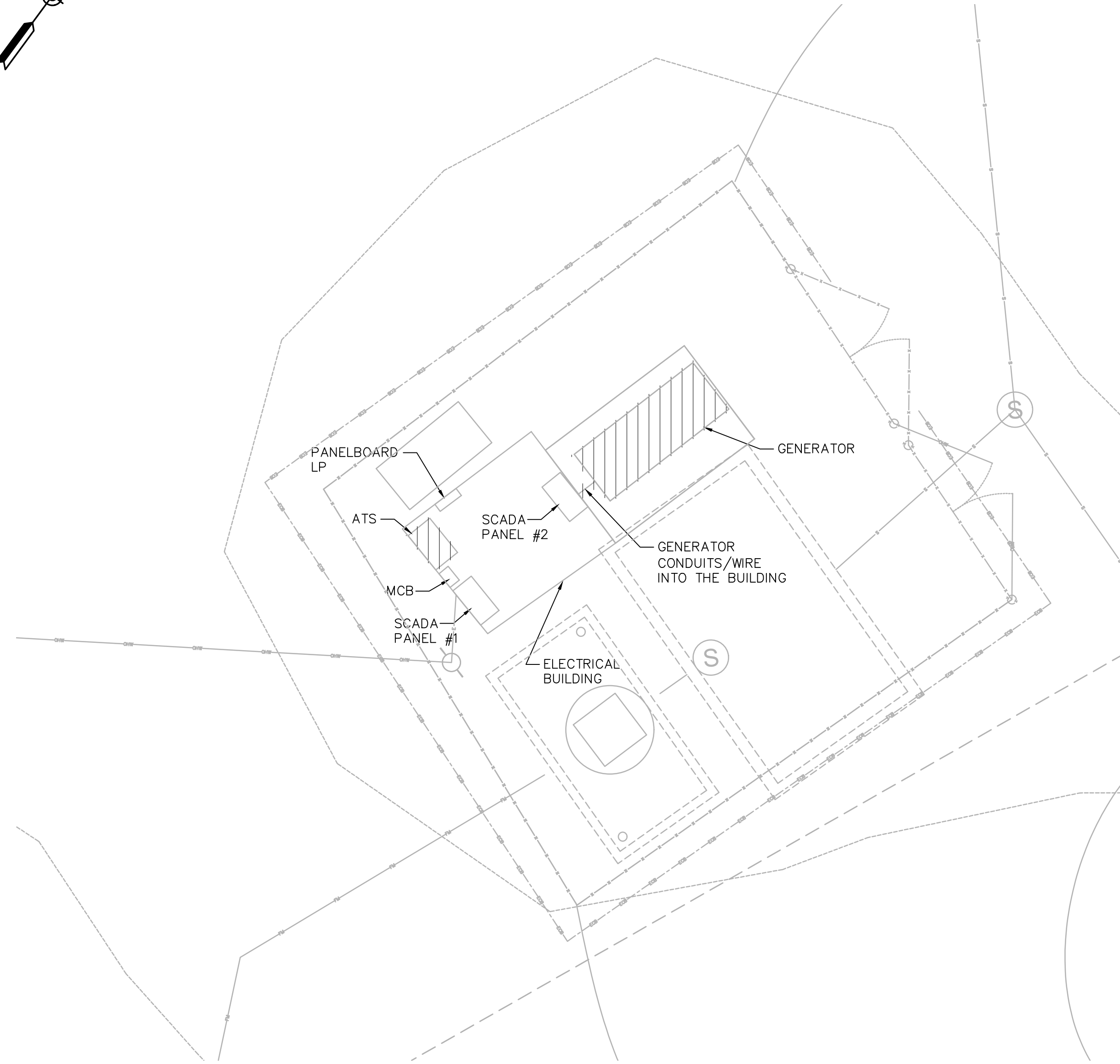
INDUSTRIAL PARK PUMP STATION DEMOLITION PLAN SCALE: 1" = 5'-0"
