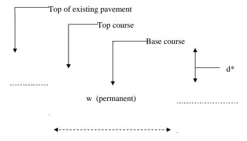
d\*= depth of existing pavement trench to a maximum of 3 inches (see general notes #3) w = maximum eligible permanent pavement width as described in paragraphs "A" & "B". equals initial width plus 2 feet and includes:
