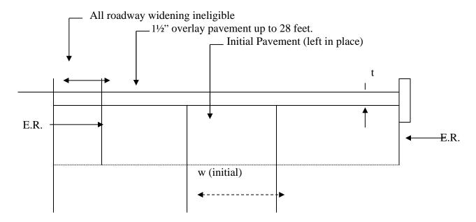
E.R.= edge of existing paved roadway t =one and one half inch (1½") overlay of bituminous concrete pavement
