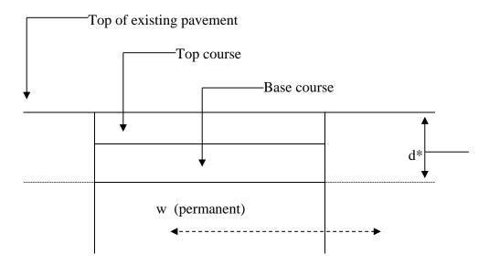
d\*= depth of existing pavement trench to a maximum of 3 inches (see general notes #3) w = maximum eligible permanent pavement width as described in paragraphs "A" & "B". equals initial width plus 2 feet and includes:
