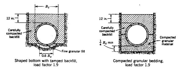
**Class B---First-Class Bedding** – Class B bedding may be achieved by either of two construction methods:
