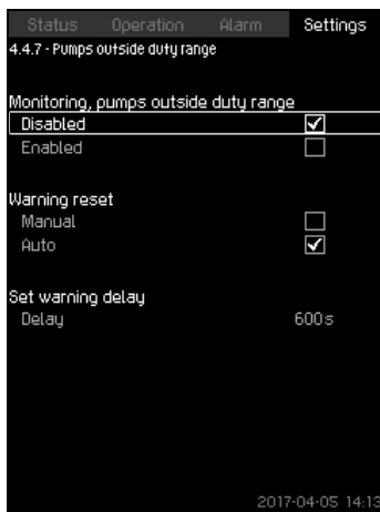
Fig. 115 Pumps outside duty range
