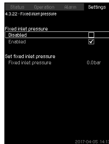
Fig. 101 Fixed inlet pressure
