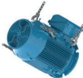
Figure 4.18 - Motor is being rotated to horizontal position
