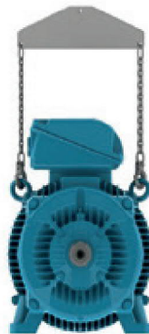
Figure 4.6 - Use of a spreader beam for lifting
