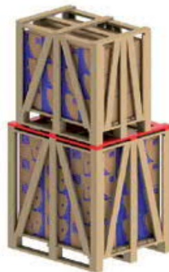
Figure 5.5 - Use of additional battens for stacking
