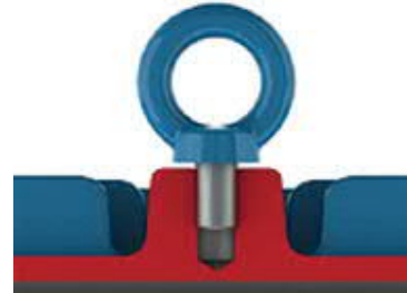
Figure 4.2 - Incorrect tightening of the eyebolt
