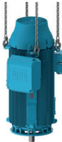
Figure 4.8 - Lifting of HGF and W50 motors.
