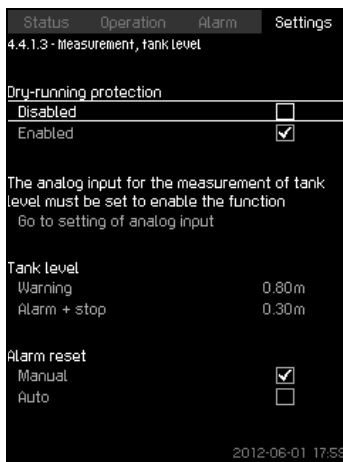
Fig. 101 Measurement, tank level
