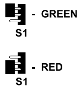
Figure 2.14 i/8D Location of S1 and Selectable Jumper Positions
