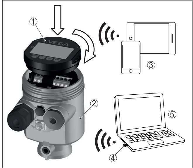
Fig. 2: Wireless connection to standard operating devices
