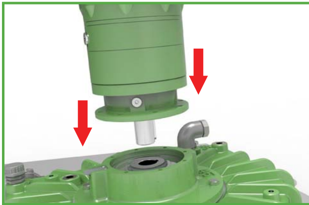
Figure 4 Installing the Gearbox
