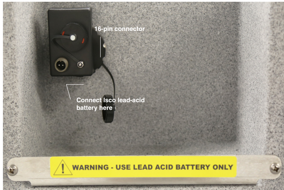
5800 battery backup module
