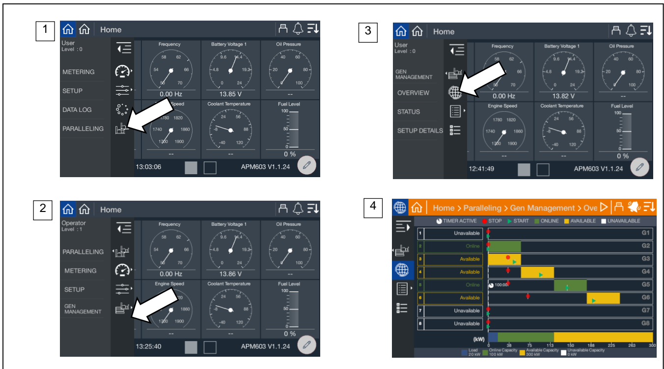
Figure 70 Paralleling Screens, Gen Management Overview
