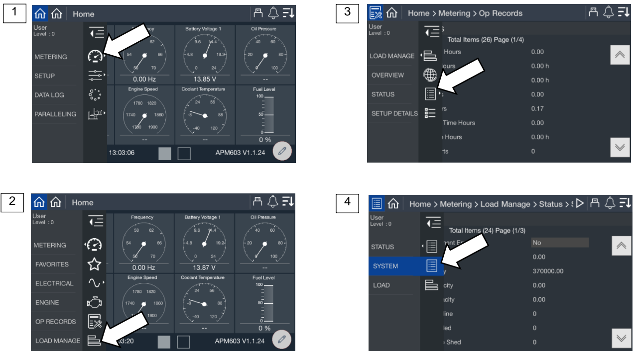
Figure 38 Metering, Load Management, Status, System
