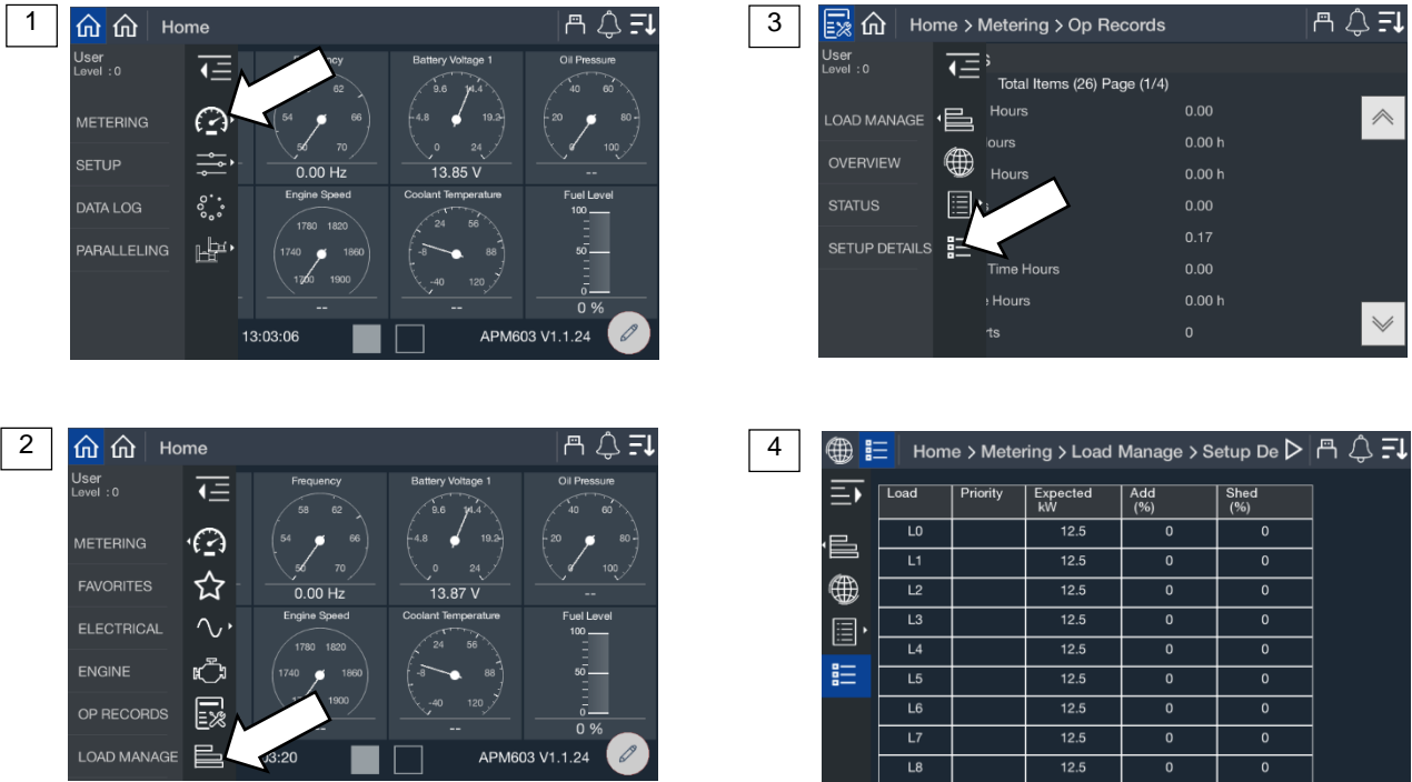
Figure 42 Metering, Load Management, Setup Details
