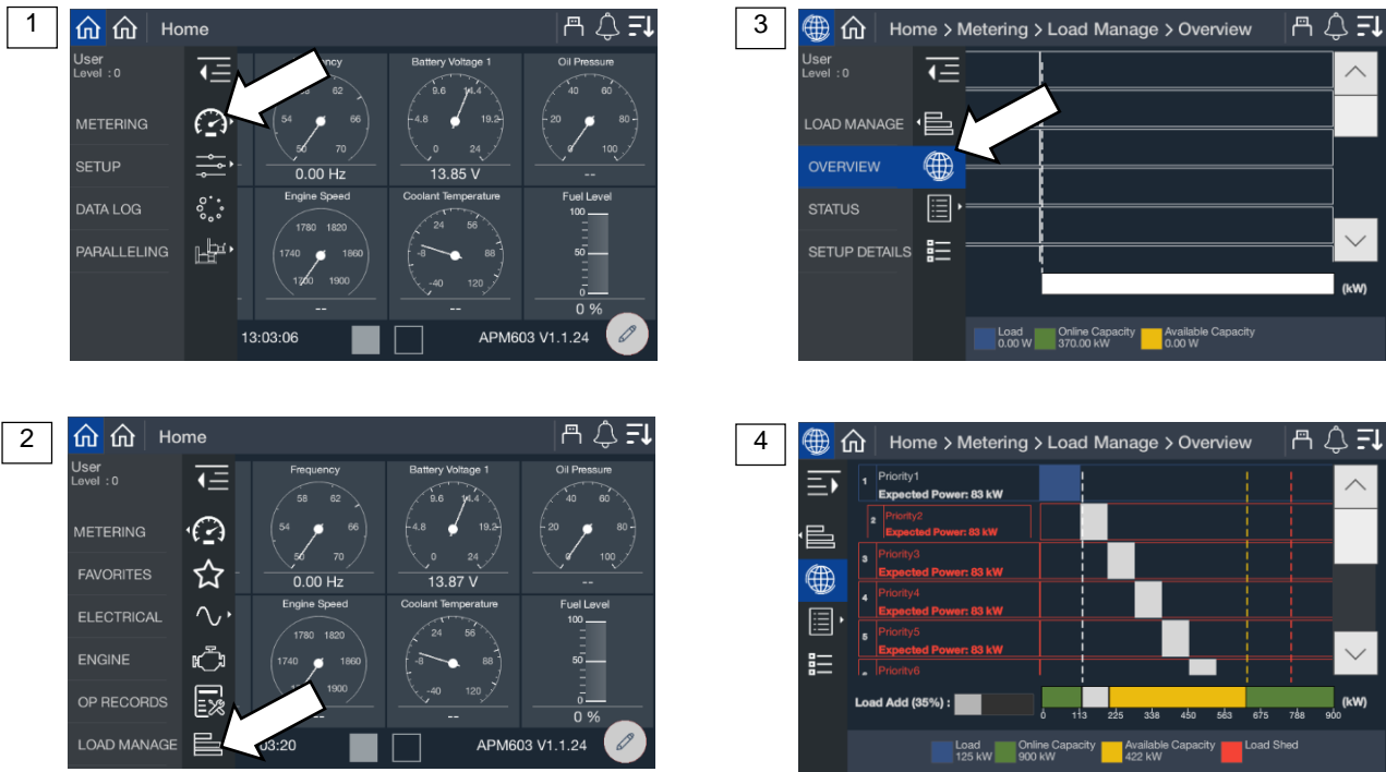
Figure 37 Metering Screens, Load Management Overview
