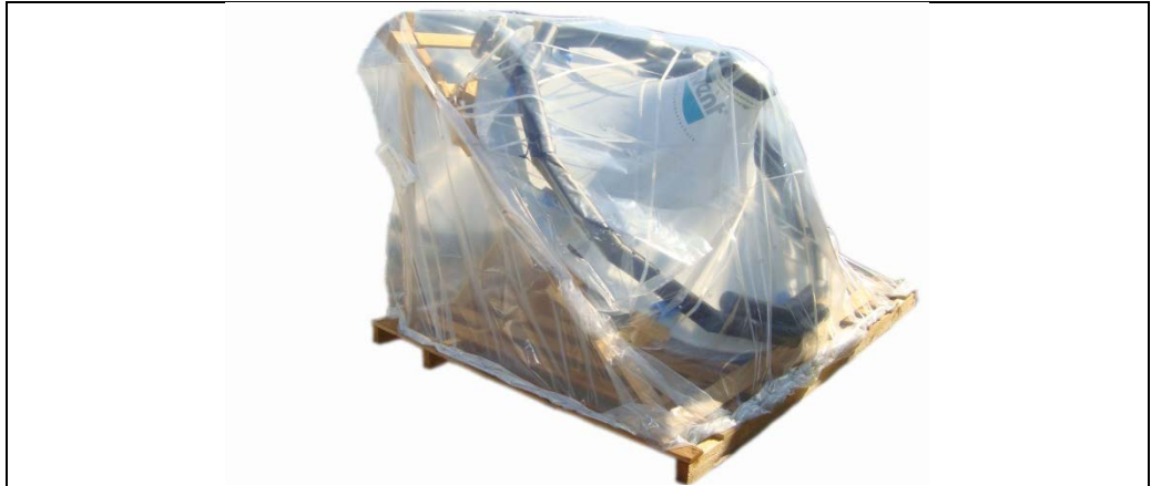
Figure 3.5: Hyperboloid Mixer body on a pallet for container shipment
