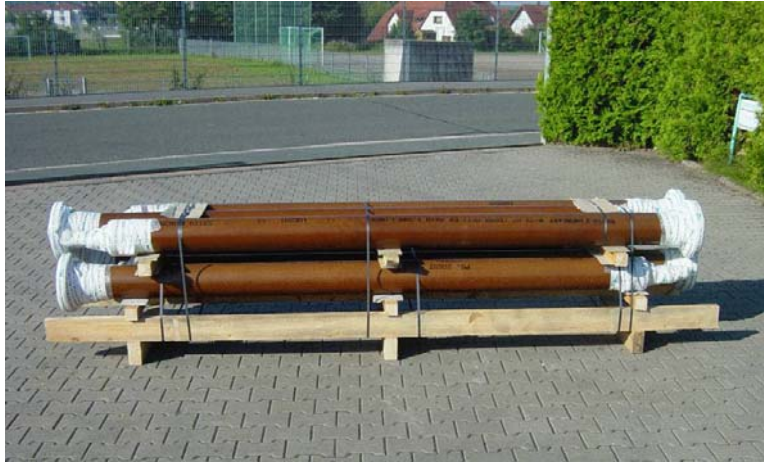
Figure 4: Storing shafts in stacks
