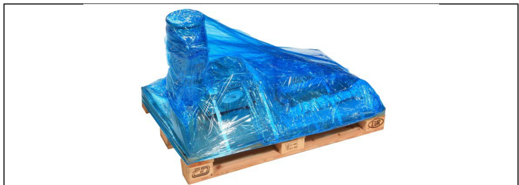
Figure 3.3: Drive unit on wooden pallet – with stretch film
