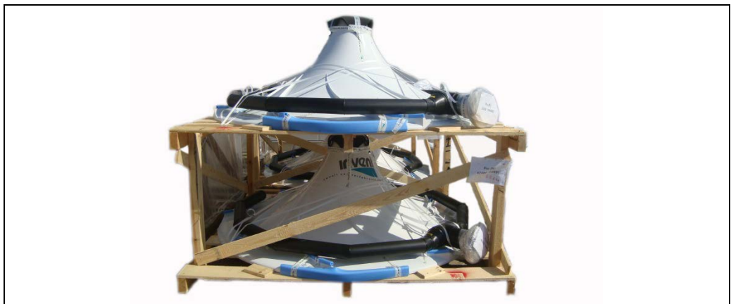
Figure 3.6: Hyperboloid Mixer body on a rack for truck transport
