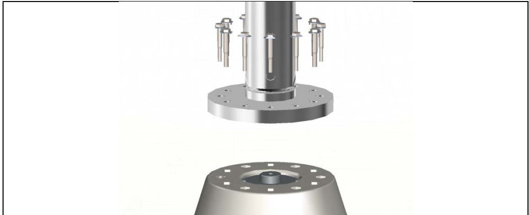
Figure 3.18: Fastening set, shaft/Mixer/Aerator body
