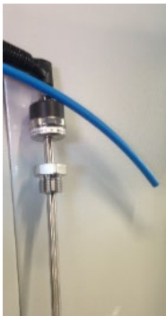
Figure 4 Temperature transmitter & plastic blue tube/pipe
