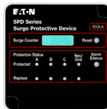
Figure 10. Standard With Surge Counter Feature Package Display
