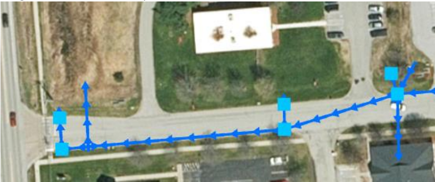
Knight Lane: Connectivity issues, no Outfalls/Outlets
